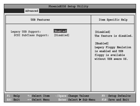
Figure 9. USB Features Submenu
